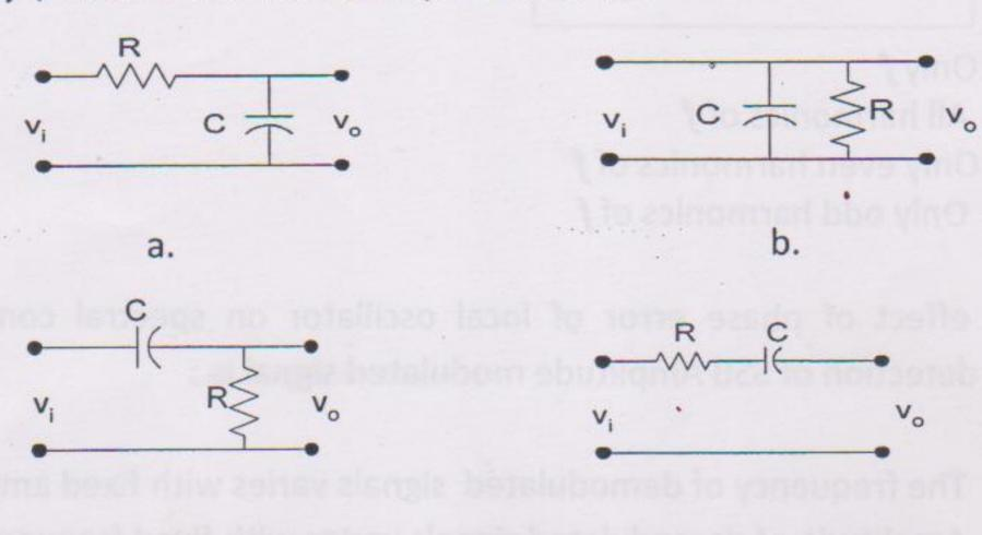
(33) For a parallel RC circuit as shown in figure, R = 20  $\Omega$  & C = 0.9 pF , which is to be matched to 50 $\Omega$  over a bandwidth,
