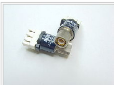
Pair of AC&E 120 \Omega twisted pair (Krone IDC) to 75 \Omega coaxial cable balun transformers. Actual length is about 3cm.
